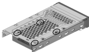
Figure 2-7. 3.5-inch Drive Carrier with 2.5-inch SAS/SATA Drive
